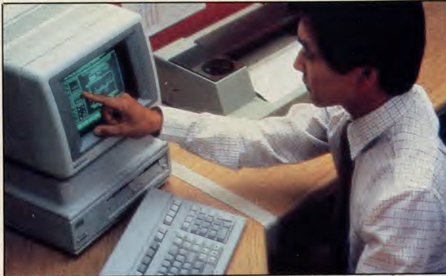
The touch screen uses a 27 by 40 grid. Any of the 1080 locations can be "read" independently of the screen display.
